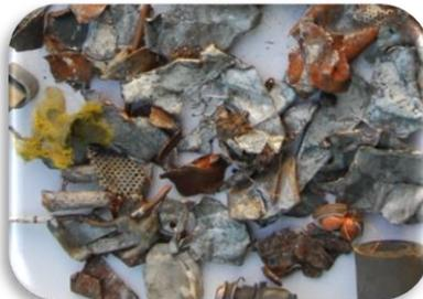
Losses of PCB to other recyclates - contamination of PCB fraction
